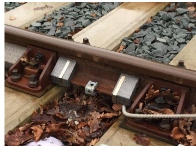
b) Insulation away from the rail temperature sensor
